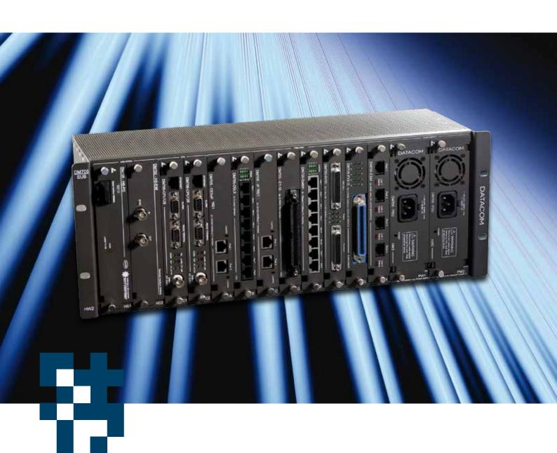
DM705 is a flexible multiservice multiplexer with access and transmission interfaces for different standards such as E1, V.35, SHDSL, FXS, FXO, Ethernet and SDH.
